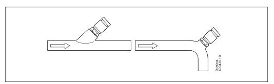
Also it is advisable to insolate the pressure transmitter from the ambient temperature or to prevent airflow around the transmitter (e.g. by motor hood).
