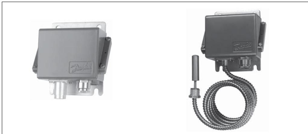
CAS units are pressure-controlled switches. The position of the contacts depends on the pressure in the inlet connection and the set value. In the series, special attention has been given to meeting demands for
